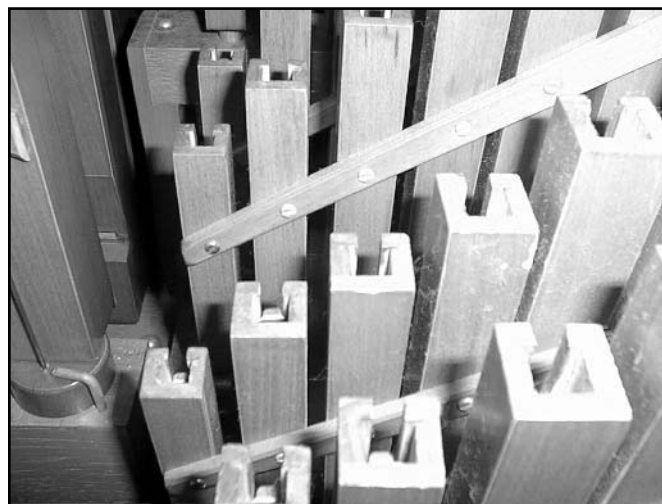
Figure 2. A view of some of the open melody pipes. Note the tuning slides.
