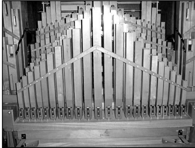
Figure 1. Seabreeze Park's Wurlitzer 165 22-note melody section. Most of the eight ranks are visible with the violins displayed in front.
